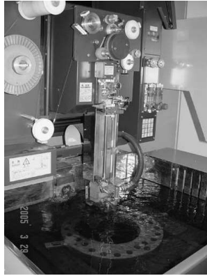
Fig. 11. Noncircular gear manufacturing using electron discharge machining [39]
